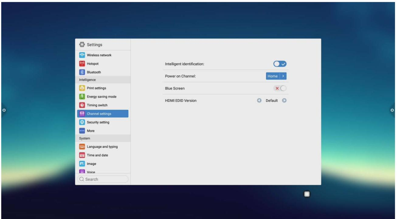
Intelligent recognition: when intelligent recognition is on, the channel will automatically jump to the channel when it detects the signal
