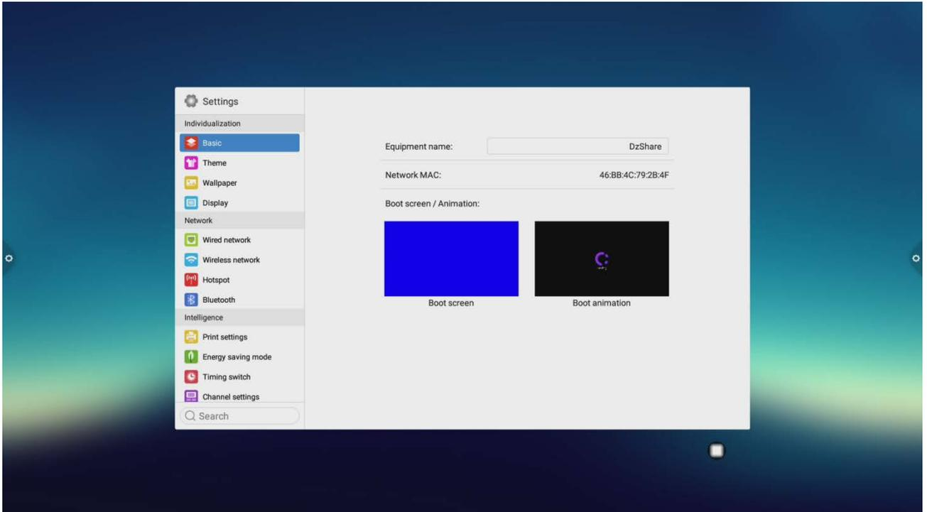
Device name: displays the current name of the machine, and the user can customize the name of the device
